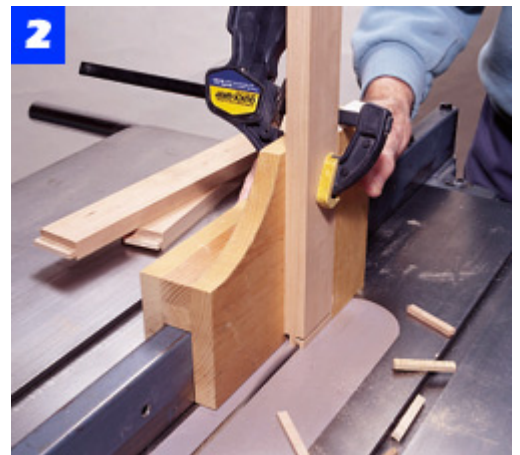
Make the tenon cheek cuts with a tenoning jig. This shopmade version slides along the table saw fence.
