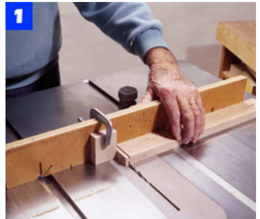
Use a stopblock clamped to an auxiliary miter gauge fence to accurately position the tenon shoulder cuts.
