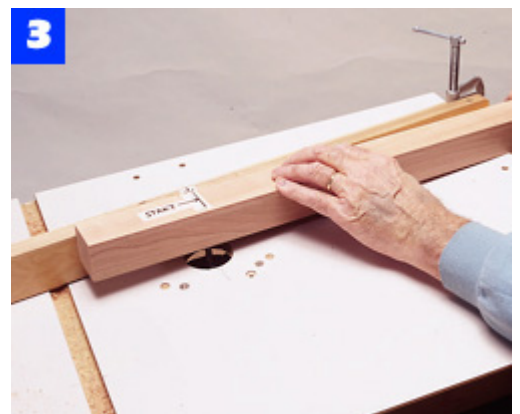
To begin a stopped groove at the blind end, lower the leg onto the bit. Then, slide the work toward the left.
